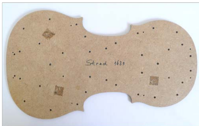
Figure 1: Inside template of the base model.
